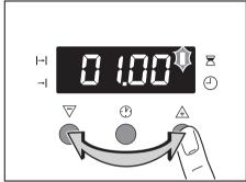
After approx. 5 seconds the display shows the time remaining. The function indicator Countdown
